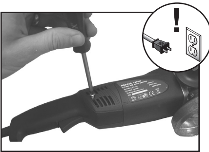
Figure 16. Removing the T10494 and T10495 brush covers.
